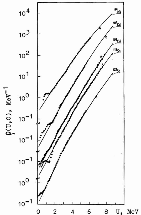
Fig.1. Energy dependence of absolute level density  $\rho(U, 0)$  for nuclei  $^{94}\text{Nb}-^{122}\text{Sb}$ . The dots stand for experimental level densities reconstructed from (p,n)-reaction neutron spectra. The solid curves for  $\rho(U, 0)$  calculation with the parameters  $\tilde{\alpha}$  and  $\Delta_0$  obtained from analysis of experimental level densities. The circles for  $\rho(B_n, 0)$  level densities corresponding to the data on neutron resonances.
